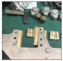
decide to make these from SAE 660 bronze which has the benefit of being good for bearing surfaces and relatively easy to machine. I could only get this in round bar but it machined well with the use of cutting oil. I machined four sticks with the right profile, making sure I made a drawing of the modification I had made for future reference if needed, and got four horn guides out of each stick. After drilling the holes and filing the radius to suit the bogie frame I trial fitted these
